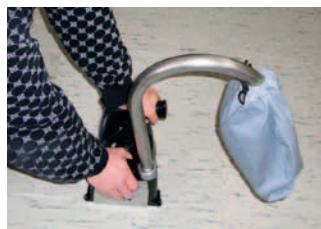
The reliable grooving machine to cut welding grooves into all different types of floor coverings without dust.
