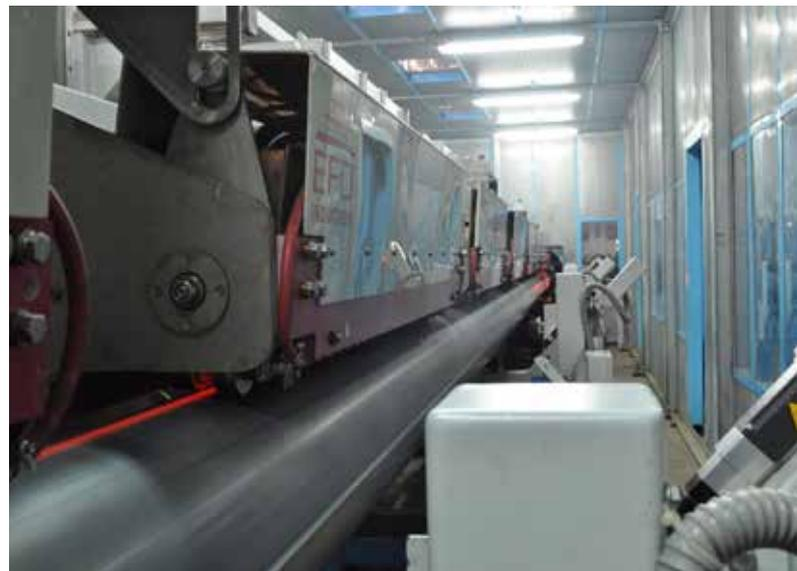
*One of our horizontal tracking seam normalizing systems. The induction coils are positioned above the pipe, and track the seam with the help of a specially designed tracking camera.*
