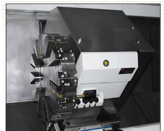
Fig. 42 Hydraulic type turret w/standard disc
