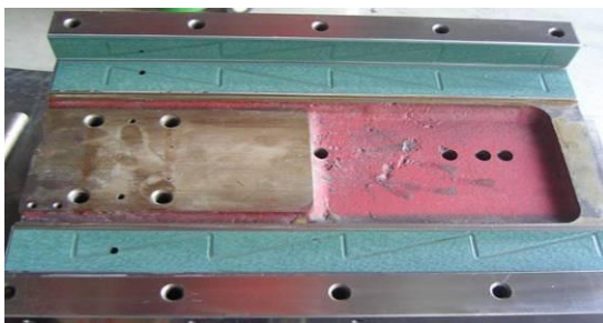
Fig. 41 Carriage plated with Turcite B
