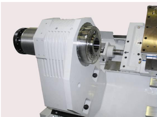
Fig. 32 Heavy cutting duty headstock
