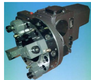
Fig.59 TBMA turret w/live tooling
