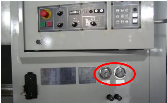
Fig. 36 Hydraulic pressure switch, hydraulic gauge and chart position
