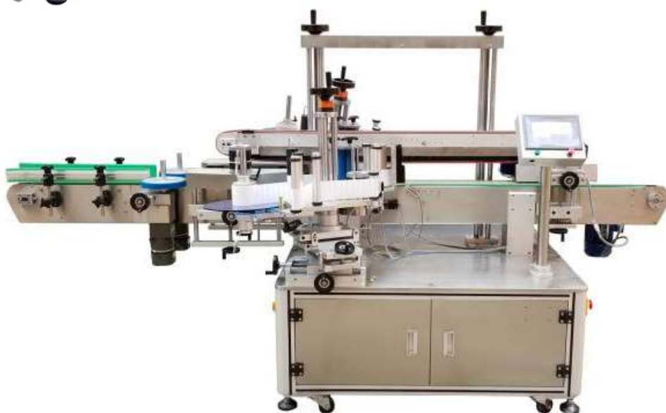
Automatic labeling machine for round bottles (1 label) and square bottles (2 labels) in action:
